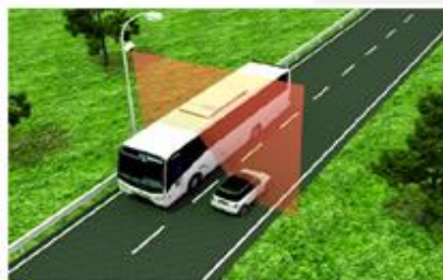
Figure 1: Installation transversale latérale
